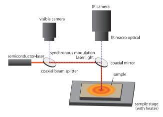
This device has allowed to detect abnormal parts in the sample and visualize the thermal properties of inhomogeneity by detecting the change in the infrared radiation amount with the infrared camera while applying the modulation cycle heating by laser to the sample.
