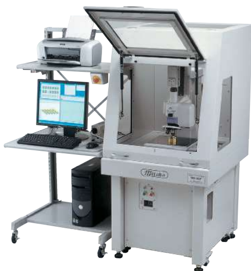
Model: NH-3SP (Super precision model) Measuring range: XYZ = 150mm X 150mm X 10mm Scale resolution: XYZ = 0.01 \mu m, 0.01 \mu m, 0.001 \mu m Applications: aspherical lenses, semiconductors, precision molds, etc.
