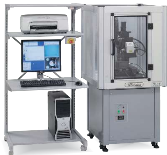
Model: MLP-2 (360-degree measurement model) Measuring range: XYZ = 120mm X 90mm X 130mm AF (R) = 40mm, AZ ( \theta ) = 360° Scale resolution: XYZ = 0.1 \mu m, 0.1 \mu m, 0.1 \mu m AF (R) = 0.01 \mu m, AZ ( \theta ) = 0.001° Applications: precision gears, endmills, punches, molds for connectors, etc.
