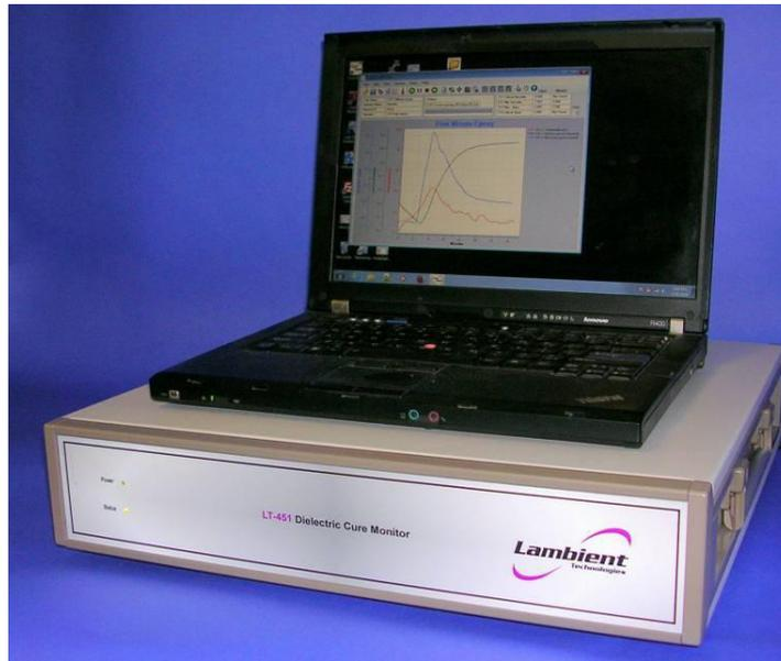
The LT-451 Dielectric Cure Monitor is a compact, versatile instrument designed for Research & Development, Quality Assurance/Quality Control, and Production applications involving the most materials—resins, composites, paints and coatings.
